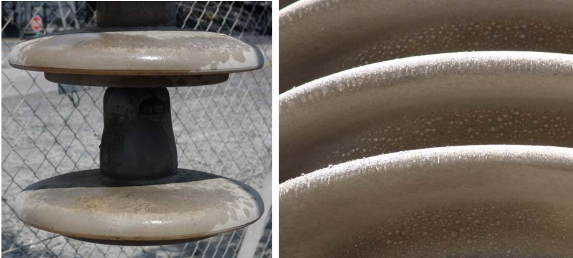
Figure 8: The hydrophilic dust-covered glass surface compared to the hydrophobicity of the coated ceramic.
